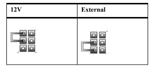
• Setting the jumpers to configure the relay position:
